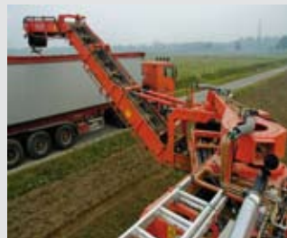
The transfer conveyor can be swung around 300° to the right or the left via two hydraulic ring gears.
